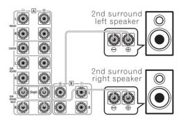
• Make sure that the + / – connections are properly inserted. (A and B speaker systems are opposite).
